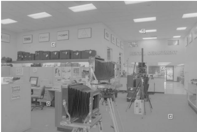
Figure 4. Image obtained by applying Debevec's algorithm on the frames from figure 2.3. Note that the image in figure 2.4 is very detailed and no region is either too dark or too bright.
